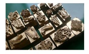
The image on the right hand side shows 'Type high dies'. There are similar to the above emojis but only larger. As such, they may not fit inside a Slip Case as such but will lock into the Chase. This thus also makes then suitable to be used with our brass type.
